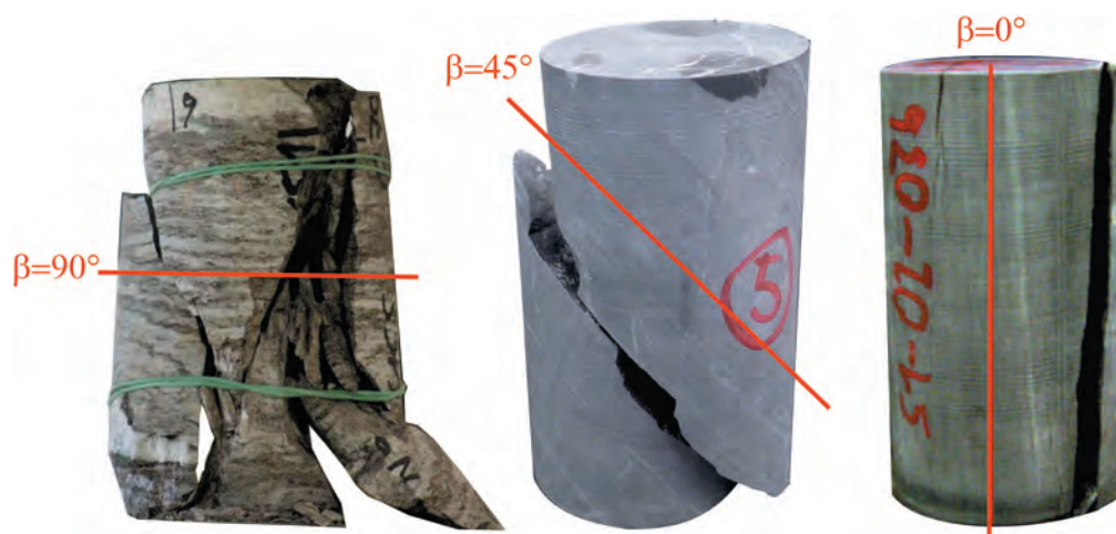
Figure 2. Examples of samples and fracture pattern in anisotropic samples.
