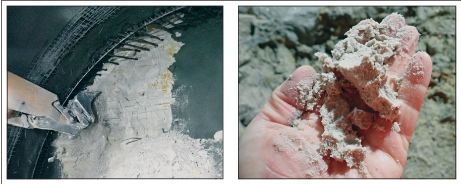
Figure 6. Typical appearance of decomposed triassic sandstone/sand of Ground Unit X1. Left image: Sequential and partial mechanical excavation in the crown section of the main tunnel. Right image: Although originally gained in form of a hand specimen, the decomposed sandstone can easily be crushed by hand
