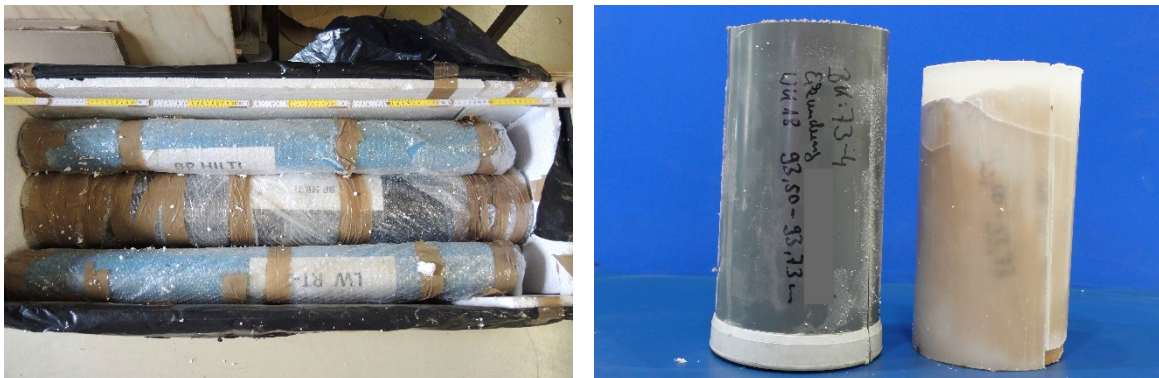
Fig. 8 Non-durable rock samples sealed in wax and in additional steel tubes (left)
