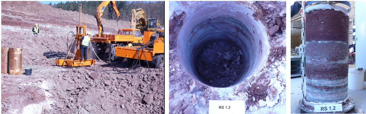
Fig. 6 Left: Coring of large diameter samples, Centre: drillhole after pullout; Right: sample after removal of tinplate
