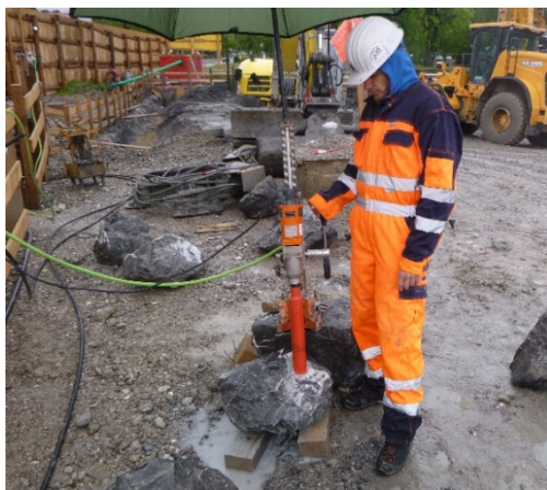
Fig. 5 Left: on-site overcoring of rock blocks in order to gain orientated samples; Right: Concept drawing for overcoring of a larger core sample in order to gain orientated specimen of smaller diameter.
