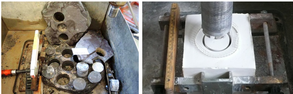
Fig. 7 Left: unsuccessful attempts to core a block sample, Right: overcoring technology with plaster embedding
