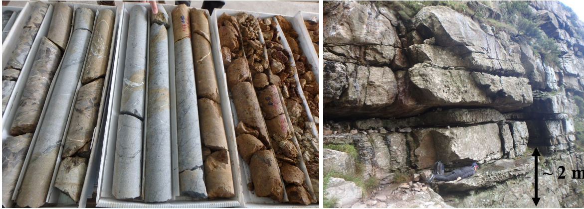
Fig. 2 Examples of identification of potential MFC left photo: core drilling indicating contact between sandstone (UCS ~ 100 MPa; low degree of fracturing) and lutite (UCS ~ 15 MPa; highly fractured), right photo: field mapping indicating potential MFC due to blockiness.
