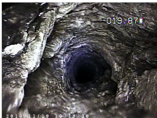
Figure 9. Example for video image in a folded quartz phyllite series in a Ø 75 mm drillhole used for ground investigation ahead of a TBM.
