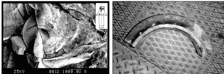
Figure 2: Left image showing shell-shaped brittle fractures in the hard metal insert of a point attack pick, about 16-fold magnification (from: [9], Figure 23, p. 23). Right image showing broken 17"-cutter disc of a hardrock TBM (Photo: Plinninger).
