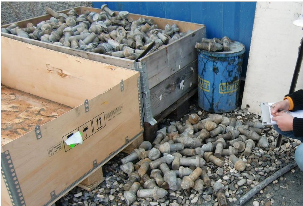
Fig. 2.1: Worn point attack picks of a roadheader, whose replacement was both caused by continuous abrasion, as well as partial failure of tool components (Photo: Plininger).
