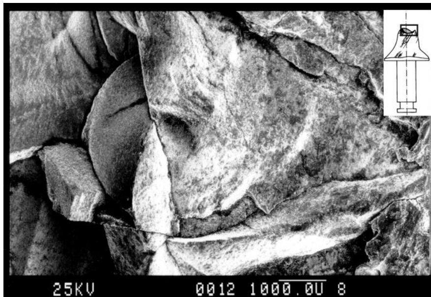
Fig. 4.1: Shell-shaped brittle fractures in the hard metal insert of a point attack pick, about 16-fold magnification. The loss of material (based on the volume of the cemented carbide insert) in this case was about 40% (from: Plinninger, 2002, Figure 23, p. 23).
