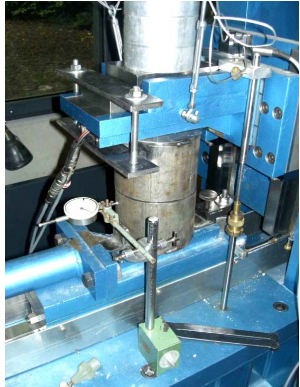
Figure 1: Testing layout of the direct shear test on model tube installations (casing-grout-combinations). Left: Scheme with internal measurements devices, right: photograph of the setup.
