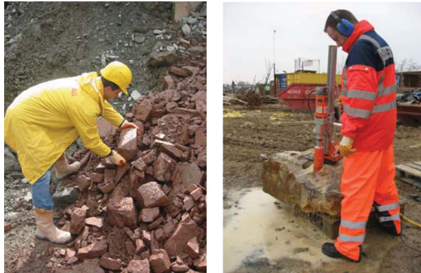
Figure 7. Sampling of fresh claystone for laboratory testing from the muckpile of a tunnel driveage (left) and overcoring of a large limestone block on site by use of a electric core drill (right).
