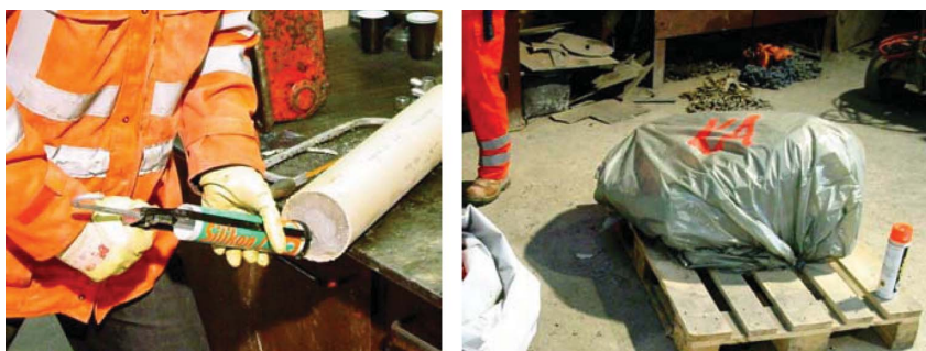
Figure 5. Examples for sealing measures for weak rock samples: Setting a silicone plug at the ends of a plastic inliner (left), simple plastic wrapping of a large block sample taken from a tunnel face (right).
