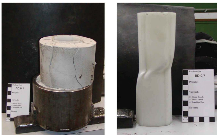
Figure 6. Specimen with type S131 ABS casing and Blitzdämmer™ industrial cement-bentonite-mixture after the shear test. Left: Complete sample after removing the upper shear box. Right: deformed ABS casing after removal of grout.
