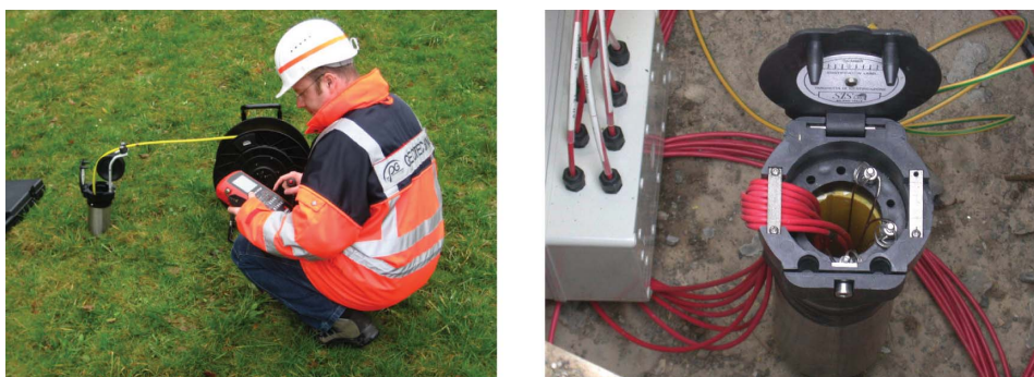
Figure 1. Inclinometer measurements using a probe inclinometer system (left) and a chain of in-place-inclinometer transducers (right; photo courtesy of SISGEO s.r.l).
