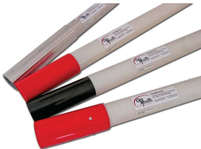
Figure 3. Examples of different inclinometer casing types, used for the investigations presented in this paper (from top to bottom): SISGEO type S111 aluminium alloy casing \varnothing 76 mm; SISGEO type S131 ABS casing \varnothing 71 mm with 3.5 mm material thickness; SISGEO Type S141 flush-coupled ABS casing \varnothing 70 mm with 5 mm material thickness and SISGEO type S151 ABS casing with 5 mm material thickness and quickjoint-system.
