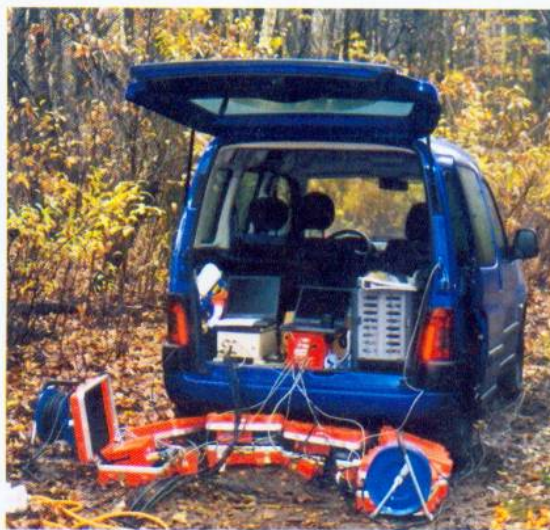
Fig. 5 Testing layout for the stability investigations using controlled vibrations.
