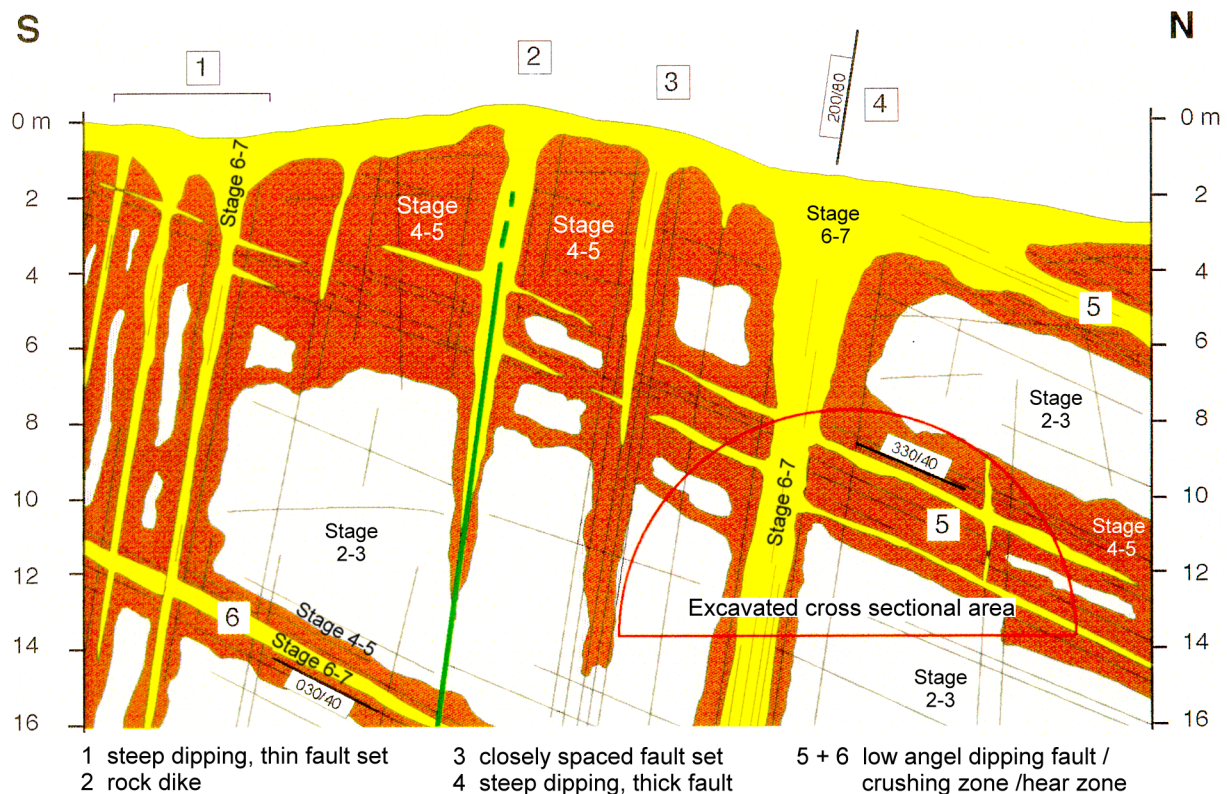
Figure 14: Model of weathering in the Königshainer Berge tunnel project with the dimension of top heading (excavated cross section area). Stages in arabic numerals refer to Figure 11.
