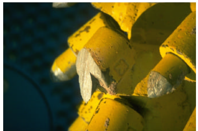
Fig. 3: Typical asymmetric wear (type 3 ⇒ Table 2) of the outer cutter head bits of the used 300 kW roadheader.
